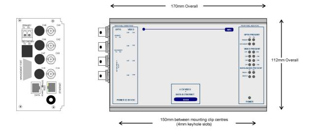
The **AMG4743BxE-SF** is a standalone four channel video transmit unit designed to transmit 4 video signals and transmit and receive up to 2 data or audio signals plus full duplex 100BaseT Ethernet connectivity over one Singlemode optical fibre.
